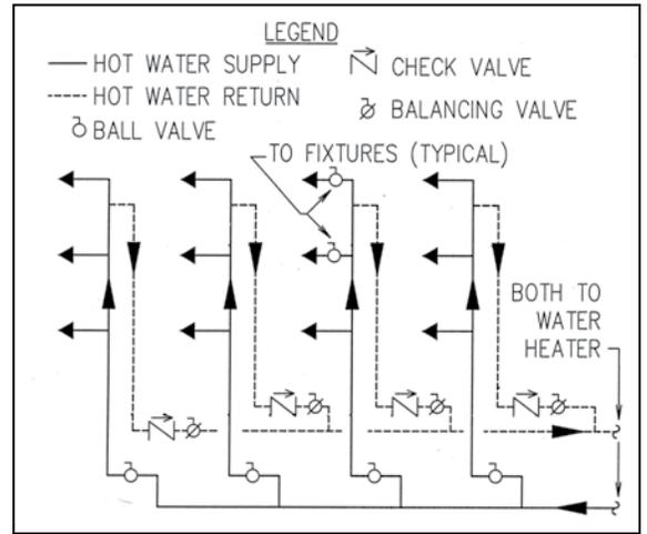
**Figure 2 Upfeed hot water system with heater at bottom of system**
