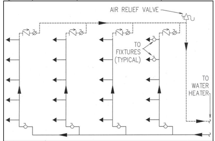
**Figure 3 Downfeed hot water system with heater at top of system**
